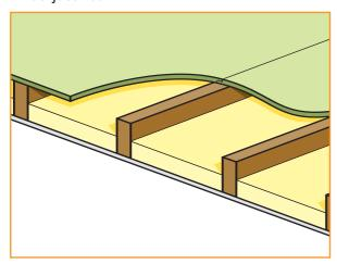
Timber floor consisting of 200mm x 50mm timber joists, with an 18mm T & G chipboard walking surface, and with 12.5mm Gyproc WallBoard TEN ceiling. APR 1200 to a minimum 100mm thickness in the floor void.
