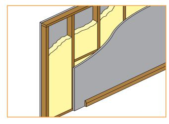
A partition wall constructed from 1 layer of 12.5mm Gyproc WallBoard each side of timber studs at 600mm centres, with APR 1200 within the cavity.
