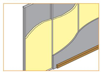
1 layer of 12.5mm Gyproc WallBoard each side of GypFrame metal studs at 600mm centres with APR 1200 within the cavity.
