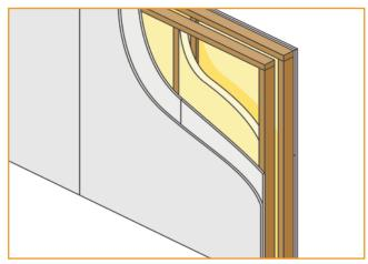
2 layers of plasterboard nominally 22Kg/m² (typically 19mm Gyproc Plank plus 12.5mm Gyproc WallBoard) with joints staggered, each side of twin timber frames with a minimum of 65mm APR 1200 in each frame.
