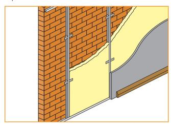
103mm brick wall with 13mm plaster on each side lined on one side with 1 layer of 12.5mm Gyproc SoundBloc board fixed to Gyproc GypLiner metal frame system (35mm gap from wall) and 25mm APR 1200 within the cavity.
