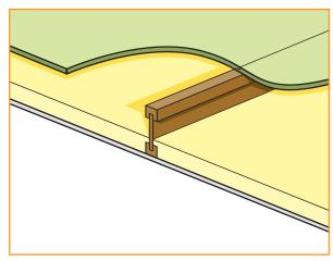
Timber floor consisting of engineered I-joists nominally 240mm deep and at 600mm centres, with a screw-fixed walking surface of 22mm T & G chipboard, and with a ceiling finish of 15mm Gyproc WallBoard screw-fixed directly to the joists. A 65mm thickness of APR 1200 laid on top of the plasterboard ceiling.
