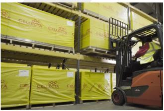
DECKfon® Quattro 39 is supplied on pallets, wrapped in temporary protection. This covering is to offer dust protection and is a temporary measure to protect the boards from the weather during the loading/unloading process, it is **not** a waterproof cover.
